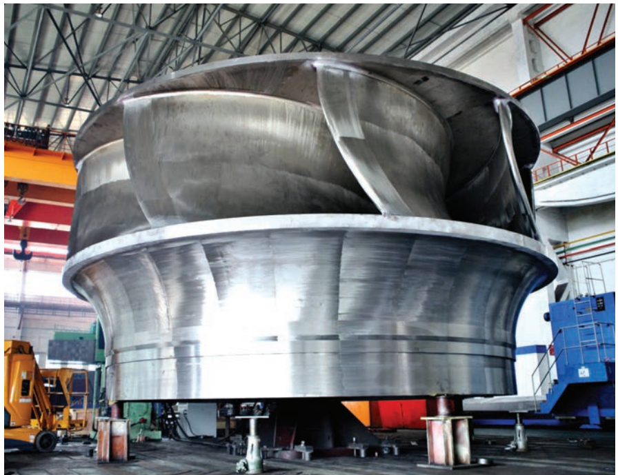
Finished, the Unit No. 1 runner assembly is a one-piece fabrication made of ASTM A487 CA6NM Class A stainless steel.
